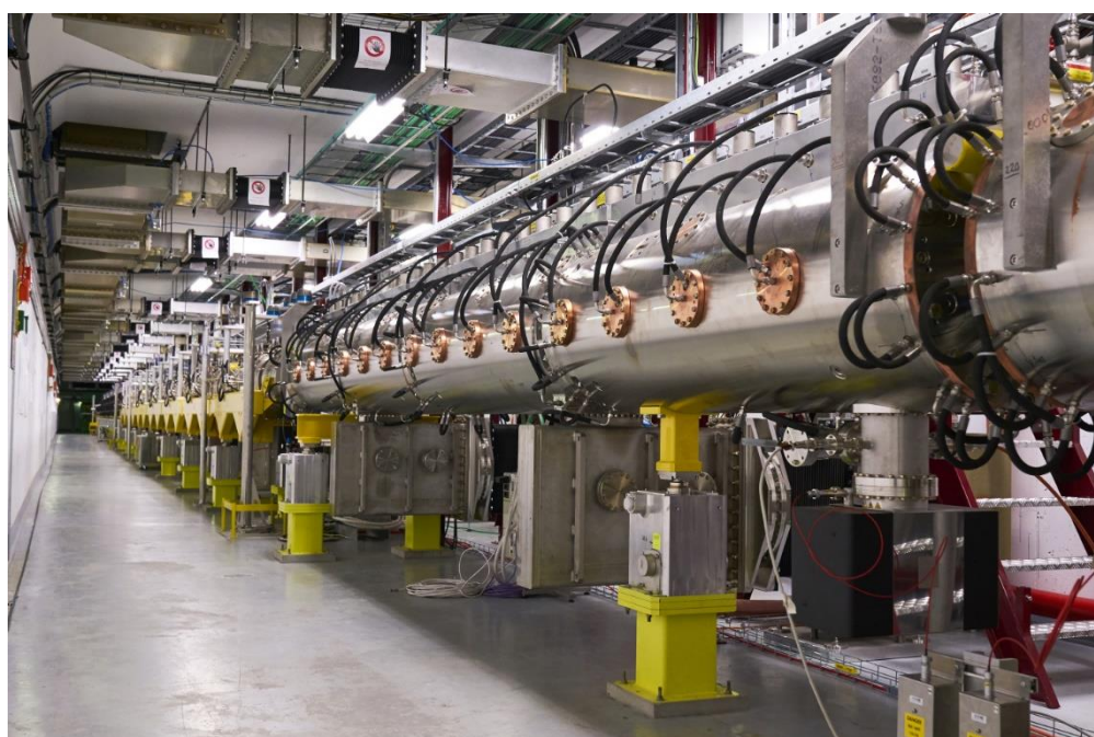
CERN's Linac4 linear accelerator is the first part of the LHC injection chain.
